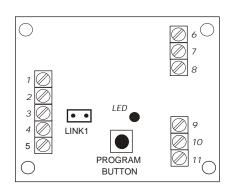
Connect trigger pins (3 and 4) to trigger, hold together for repeat-triggering With LINK1 fitted, the timing cycle will complete before allowing another trigger. With LINK1 removed, the timing cycle can be re-started by re-triggering and the timing cycle will not start until the initial trigger goes open circuit.
